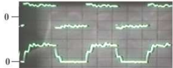
Fig.20 Stator voltage & Stator current Horizontal: Time 20 ms/div & Freq. 25 step/s Vertical: Upper Trace (Stator voltage) 10 V/div Lower Trace (Stator current) 0.2 A/div
